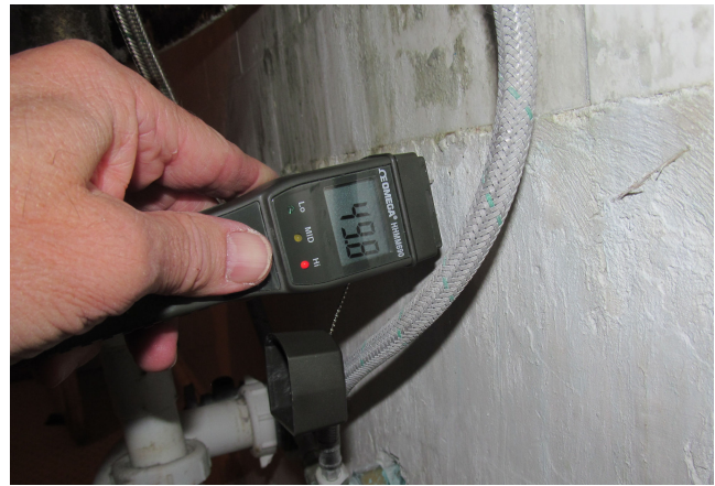
Figure 2. A moisture meter being used to detect hidden leaks in a kitchen. Access to moisture is crucial for German cockroach survival, making routine inspections essential for effective IPM programs in multi-unit housing. Photo credit: Herb Field
